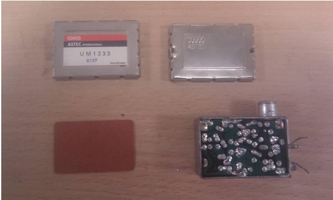
Figure 4: The UHF modulator with bottom and plastic insulator removed
