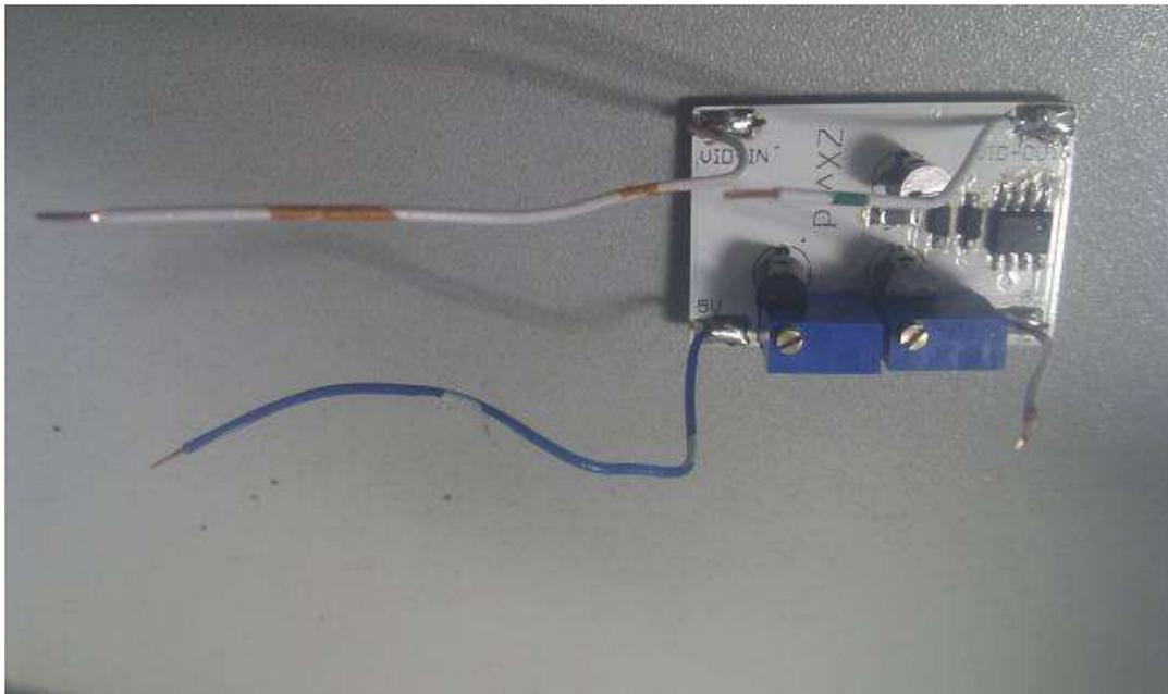
The bare unit comes with four wires which need attaching to your ZX81.
