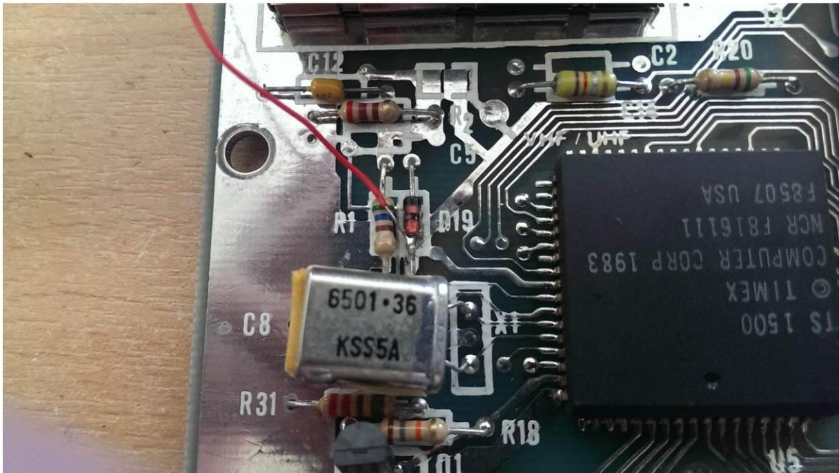
Figure 10: Showing the VID-IN connection to D19 on the T/S 1500
