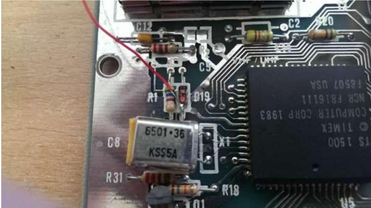
Figure 10: Showing the VID-IN connection to D19 on the T/S 1500
