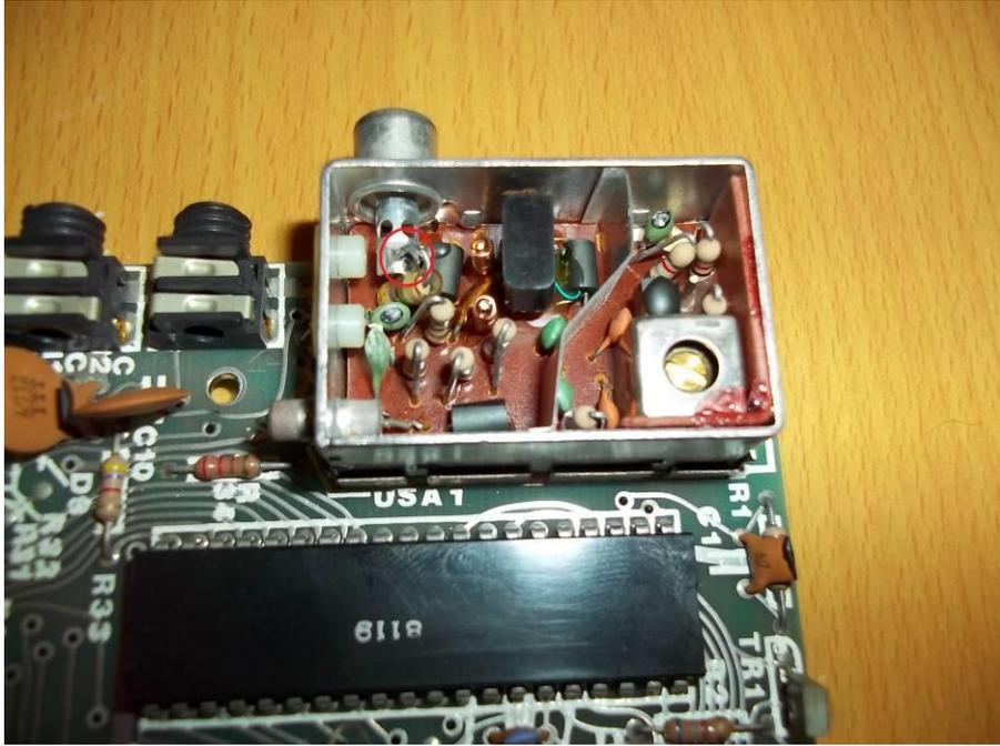
Figure 2: The inside of the TV modulator - this will all be removed!
