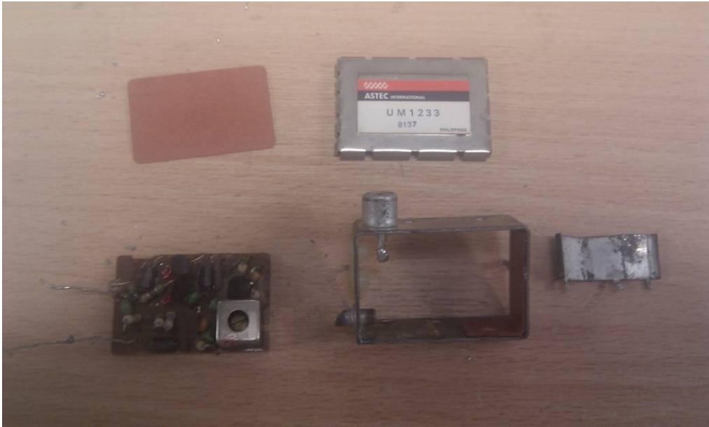
Figure 5: The UHF modulator once stripped out ready to accept the ZXvid
