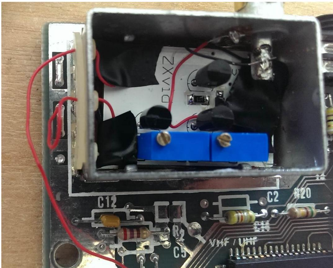
Figure 9: The ZXvid in place - showing the +5V and VID-IN connections
