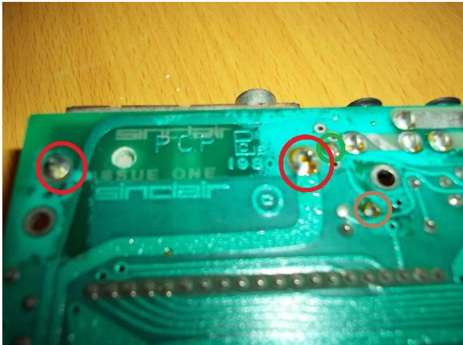
Figure 3: The solder points for the UHF modulator and feed wires
